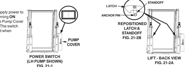
If possible, apply power to the Lift by turning ON switch on the Pump Cover (FIG. 21-1). The switch is illuminated when turned **ON**.
